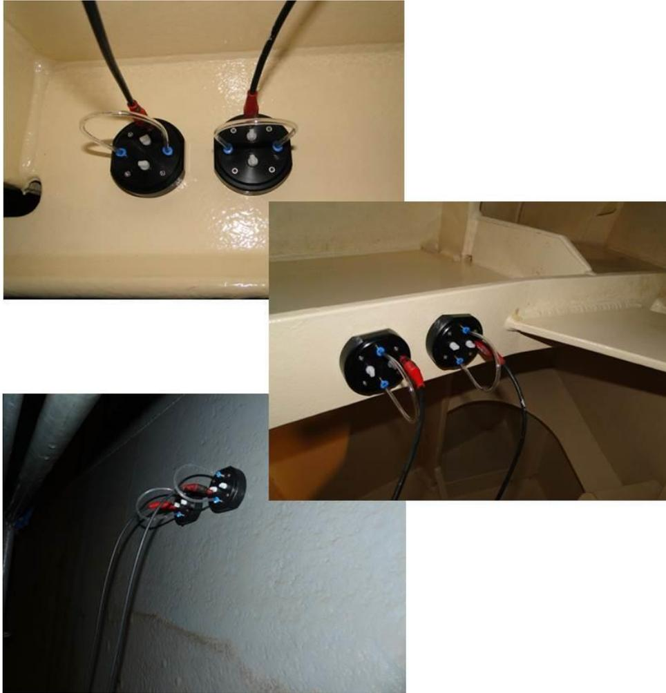
*Figure 19: MCF Cells used during measurements in a ballas tank, bulk head, drinking water tank. [Photo's courtesy of ENDURES]*
